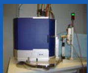
STOE powder diffraction system LaB 6 powder sample / capillary ∅ 250 µm time: 3 min / image plate detector
