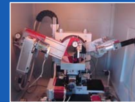
experimental setup: Diffractometer XRD 3003 (Gö-1) for samples up to 200 mm × 200 mm or 8" ∅ and for measurements up to 2θ = 160°
