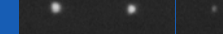
Symmetric shape of secondary focal spots with ∅ < 100µm up to ∅ > 300µm measured at fixed anode tubes (Cu) coupled with ASTIX-f (marcam images)
