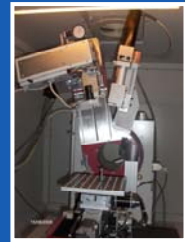
experimental setup: Diffractometer XRD 3003 (Gö-1) for samples up to 200 mm × 200 mm or 8" ∅ and for measurements up to 2θ = 160°
